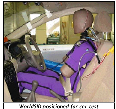
WorldSID positioned for car test
