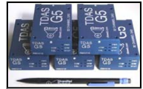
WorldSID Data Acquisition System, 160 data channels
