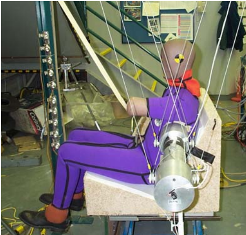
ISO TR9790 pendulum test on WorldSID
