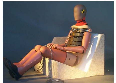
WorldSID prototype with jacket removed
